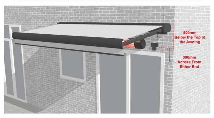
(x3) 13amp outlets are required which can either be: (x3) BG Storm 13A Weather-proof Switched Fused Spur OR (x2) MK Masterseal Plus 13A 2 Gang Switched Socket.
