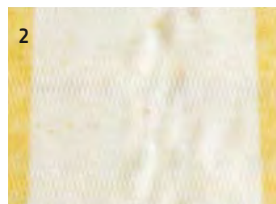
Winding creases in the centre of the awning fabric
