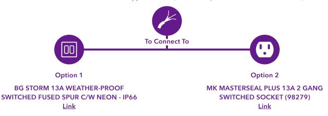
(This is what we require from the electrician, so once we come to install the product it should be ready for us to connect. Please note this is a guidance link only. The waterproof switch will be determined by the customer.)
